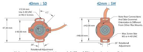
All dimensions are in mm with a tolerance of ±0.127 or ±0.254 unless otherwise specified.
