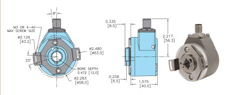
All dimensions are in inches with a tolerance of +0.005" or +0.01" unless otherwise specified. Metric dimensions are given in brackets (mm)
