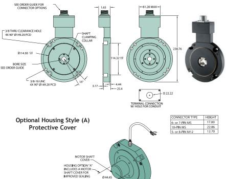
All dimensions are in mm with a tolerance of  $\pm 0.254$  unless otherwise specified
