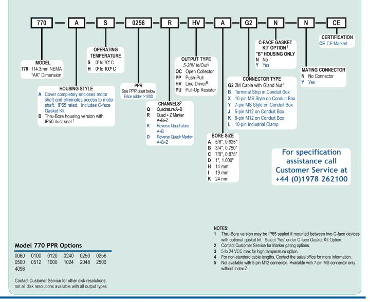
Incremental Thru-Bore Motor Mount Encoders
